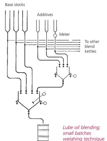
If the blending plant building height allows, cascade blending can produce very accurate batches, very quickly with a minimal risk of contamination. Base components can be metered/weighed into a 'kettle' before pre-mixing (cocktailing) which can be flushed clean to avoid contamination.
