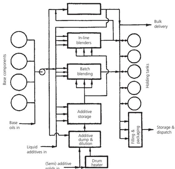
are discharged to storage, to filling machines or despatched in bulk. The laboratory checks this entire process from start to finish to ensure quality.
