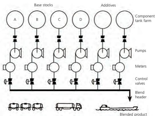
Each component/base stock stream is accurately controlled and the blend header discharges a final blended product that is correct from start to finish.
