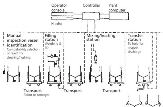
This type of system (shown above) requires a purpose built plant and tends to limit the batch size to about 5 tons, due to transport considerations. If used in conjunction with load cells (with an accuracy/linearity of 0.04% over 10 to 1 range) the small volume additives may have to be pre-mixed by cocktailing or dilution before the final process.
