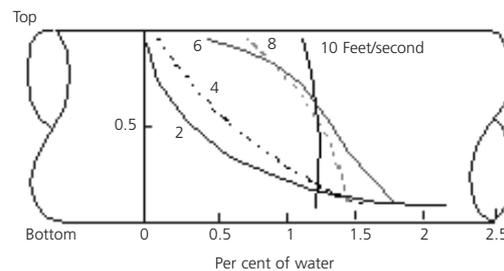
Figure 6. Concentration vs. velocity in horizontal pipes
