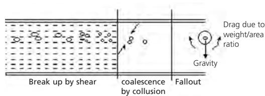
Figure 2. Droplet break-up and coalescence
