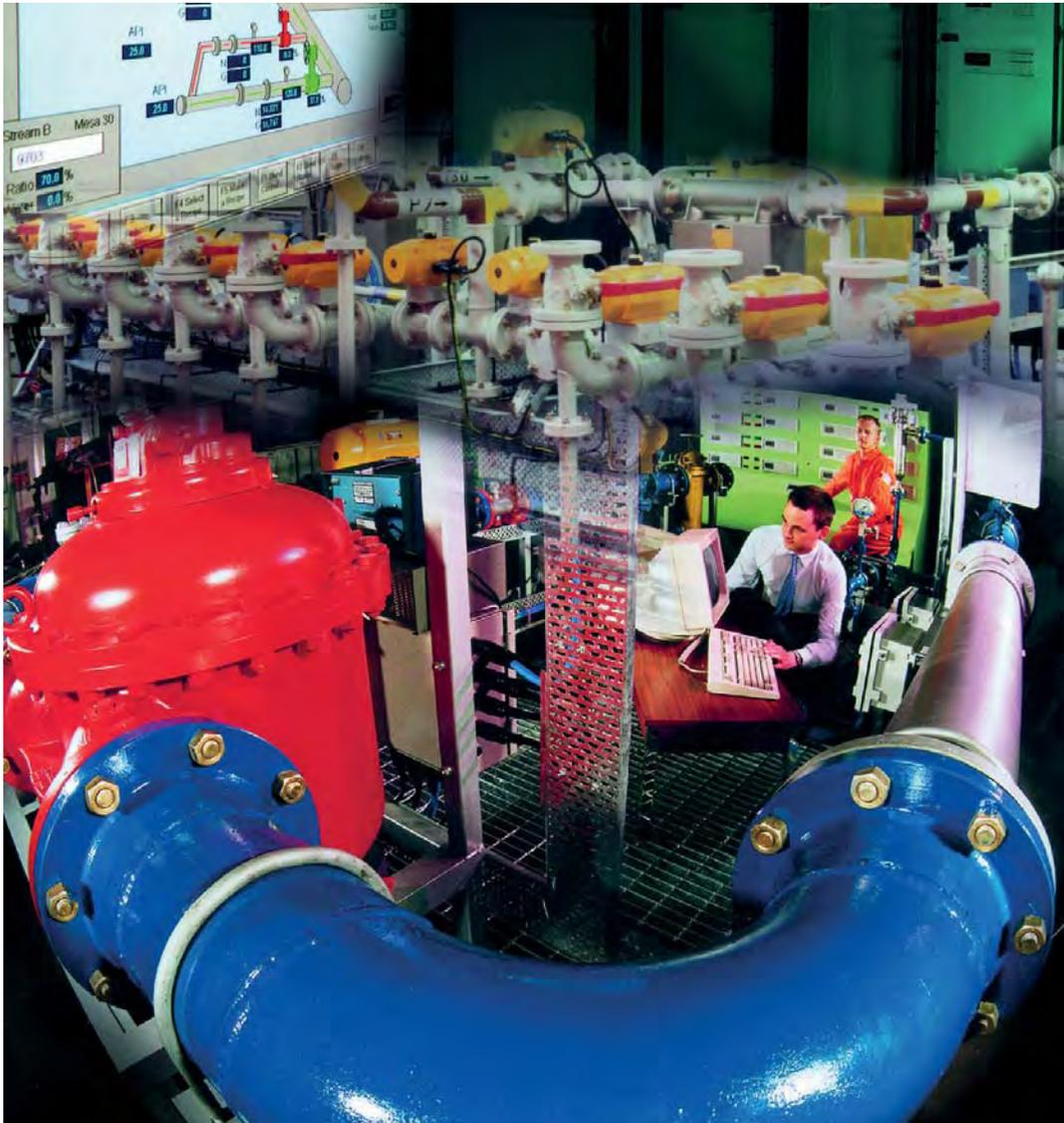
In-line blending is the controlled, continuous mixing of a number of components to produce a finished product of closely defined quality. The quality of the product is controlled as it is made. This is invaluable in continuous process industries because the final product can be blended, analysed and loaded in a single process.
