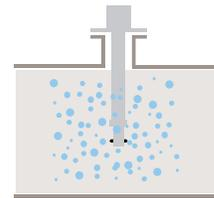
*Small sample probe entries can only cope with small water droplets*
