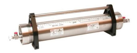
Cameron's JISKOOT™ CPC is a range of low cost, constant pressure (variable volume) sample receivers for the receipt, storage, and transportation of liquid and gaseous hydrocarbon samples. The receivers are designed to be pre-charged with inert gas to maintain the sample at process pressure conditions for analysis.
